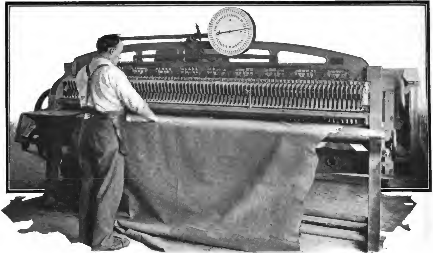
Special machine used for measuring the area of hides employed in upholstering cars in the Studebaker factory at Detroit, Mich.
